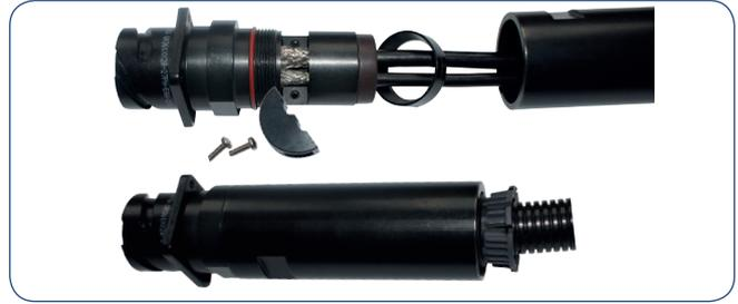
Backshell, fully rubber covered as protection against sandblast and abrasions, including a full receptacle cover. With integrated cable strain relieve and 360° shield connection against EMI impacts.
