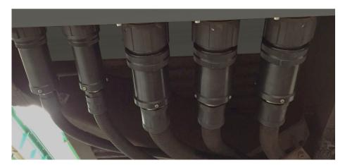
The fully assembled cable junction box on the underside of the car with the GIMOTA sliding backshell and the PMA screw connections.
